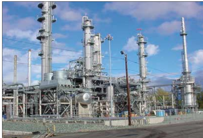
State Highway 20 travelers can see Shell's low sulfur gasoline hydrotreater from the road. The unit produces low sulfur gasoline.
